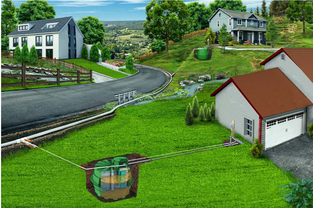
Figure 2 STEP System Schematic
